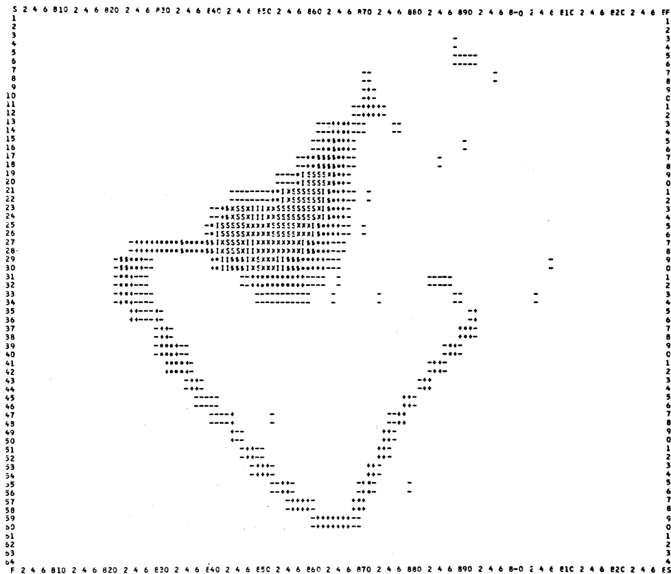
Fig. 3. Computer plotted isophotes of the lithium release obtained from the magnetic tape data for the firing of 21 June 1973. This matrix should be compared with the frame shown in Fig. 2c.
